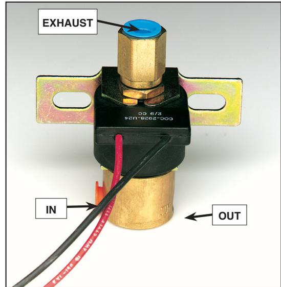
Normally Closed Valve is mostly used with Normally Open Switches on Freightliner, KW, Peterbilt, Western Star and Volvo
