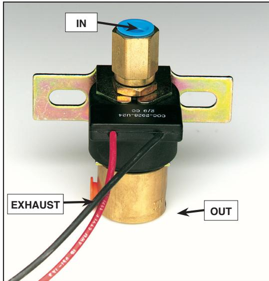
Normally Open Valve is mostly used with Normally Closed Switches on Navistar and Ford
